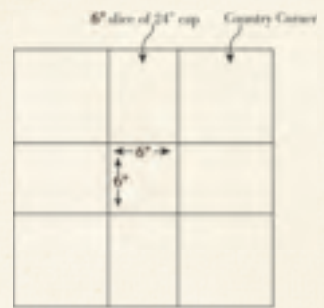
Cap for 26" Pier: Size: 30" square Note: Leave 6" square in center open for plantings or cover with 24" pier cap.
